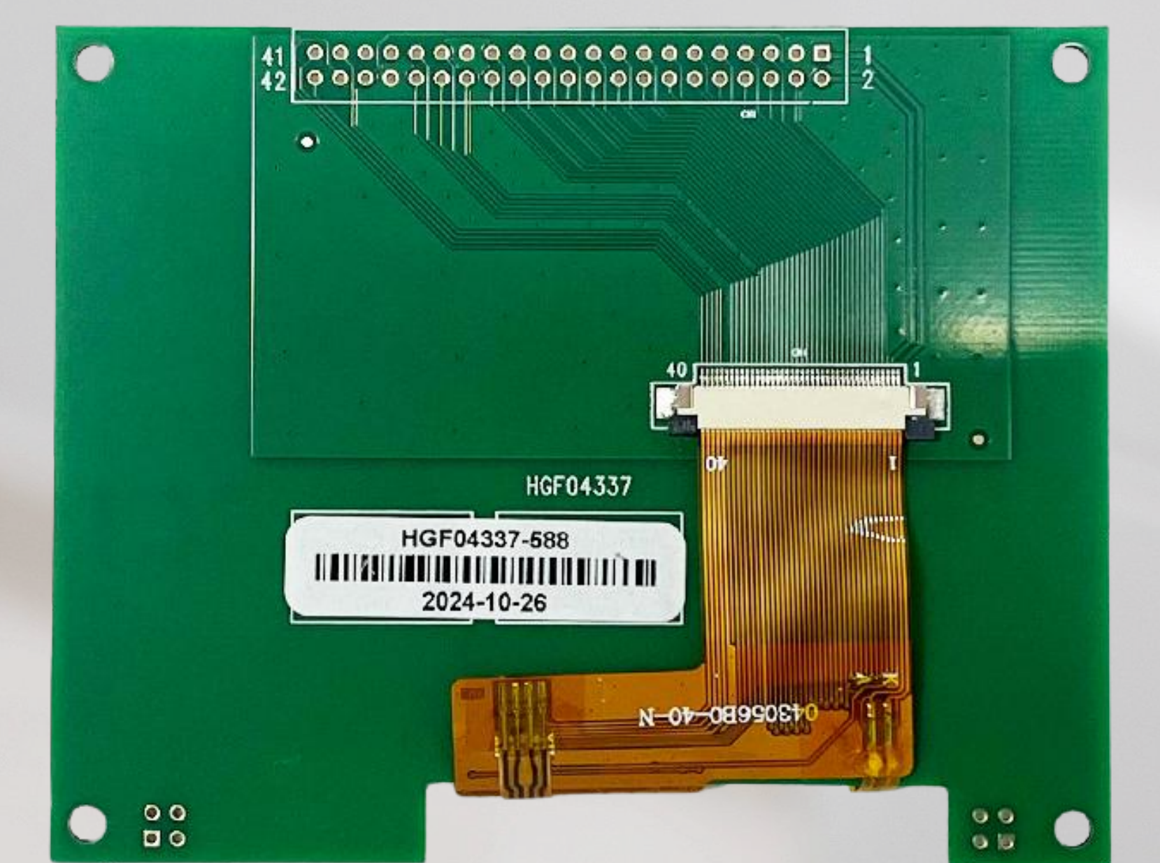
TFT and RTP integrated on PCB
